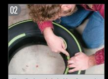
We outlined our desired whitewall area using common painter's tape. After painting, you must score around the painted edges to prevent tearing the paint upon removal of the tape.
