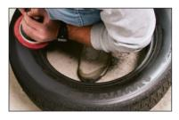
After removing the lettering, we buffed the sidewalls with 400-grit sandpaper to ensure they were smooth all the way around.
