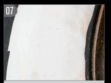
After removing the thin layer of black rubber, we noticed manufacturing imperfections around the edges of the whitewall. While these are visible up close, they are hard to see from a distance.
