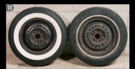
After successfully exposing the wide whitewall on our cheap used tire, we scrubbed the tire using Westley's Bleche-Wite, to remove any remaining rubber particles. The result is a wide whitewall tire that looks great and cost very little other than a bit of time with some sandpaper and bleach.
