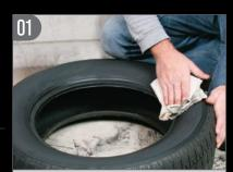
To start the process, we wiped the tire down with Westley's Bleche-Wite to ensure the tire was free of any dirt or oils. It is important to clean the tires before trying to paint them.
