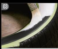
Using a brush, we applied a moderate amount of the whitewall paint to the taped off area.
