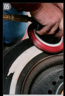
Using 180-grit sandpaper on a pneumatic 5-inch random orbital sander (ROS), we gradually removed the thin layer of black rubber.
