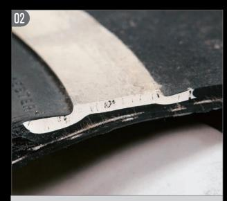
Using a junk tire, we cut through the sidewall to show just how wide the ring of naturally white rubber is on the average whitewall tire. As you can see, a very thin layer of black rubber covers much of the available white rubber. The cutaway view shows that grinding back the thin layer of black rubber will have essentially no affect on the strength of the tire's sidewall.
