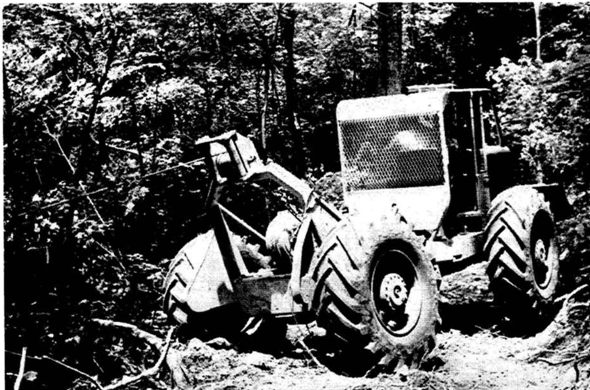
Figure 1.—A typical underinflated and overloaded tire on a log skidder. This kind of abuse leads to serious and costly damage.
