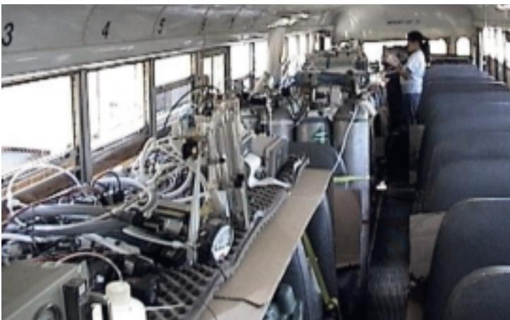
Figure 4. UCLA graduate student operating instruments on diesel school bus. (Fitz, Winer, Colome, 2003)
