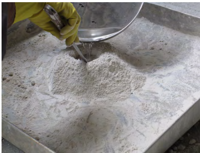
Figure 3: Mixing of Kaolin with optimum moisture content
