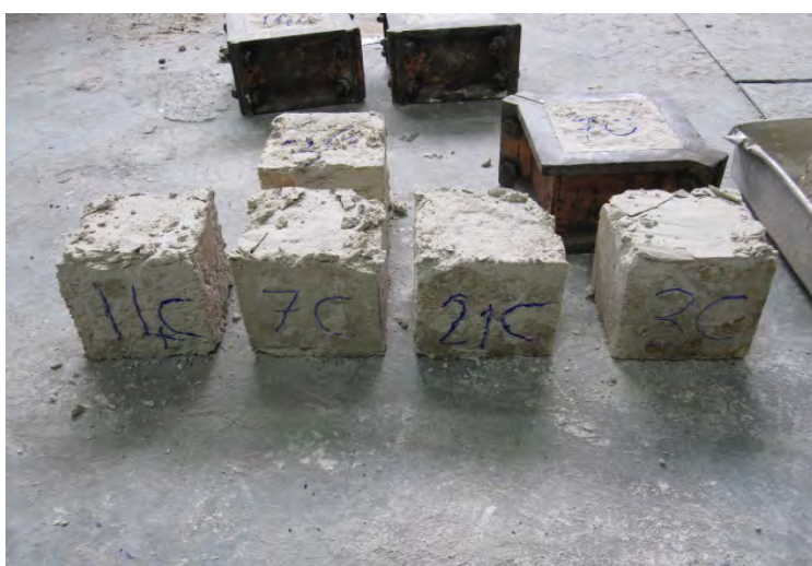
Figure 7: View of Different Cases of Concrete Particles in Compressive Test
