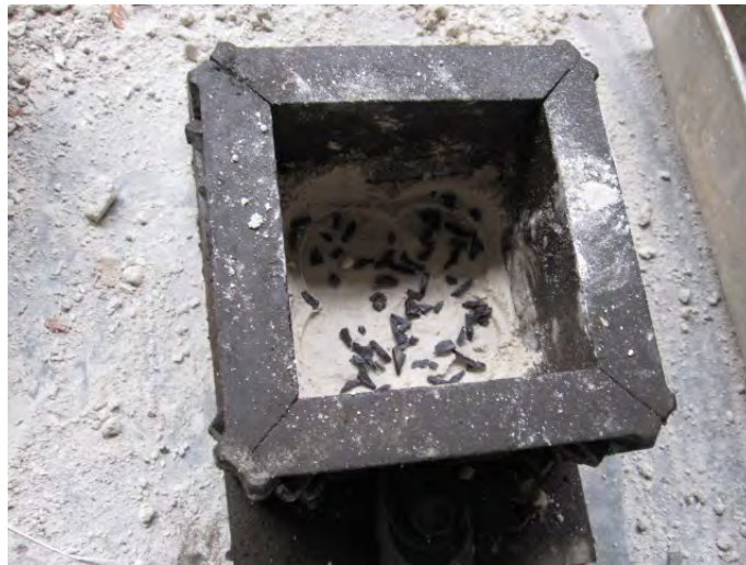
Figure 4: View of Shred tires in 1/3 Layer of Mould
