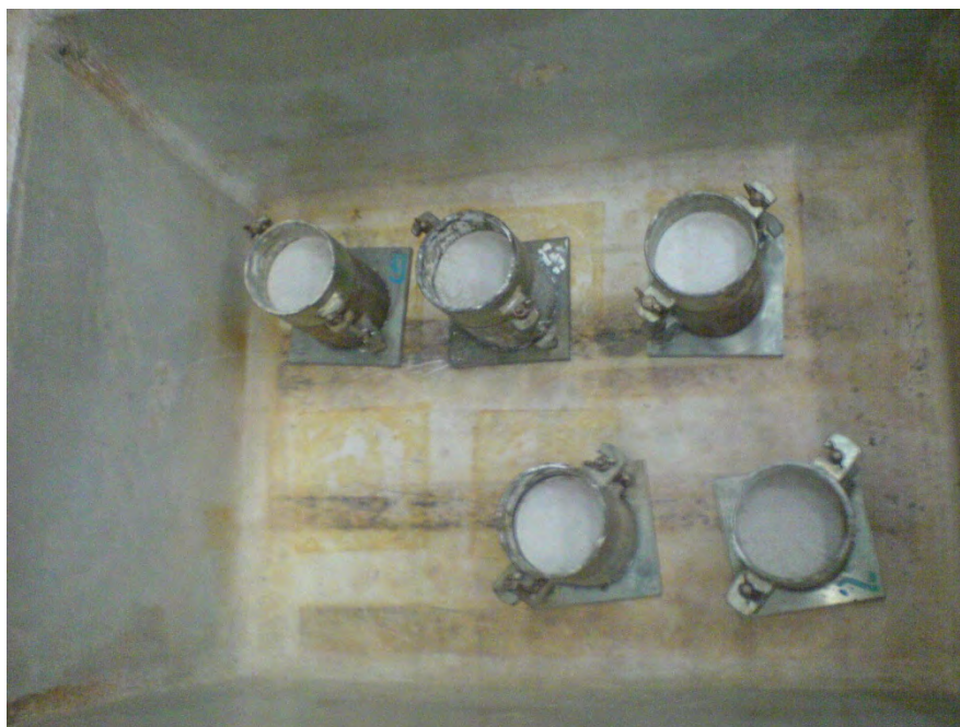
Figure 2: Compaction Test of Kaolin
